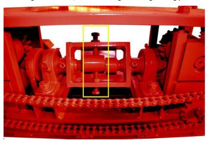
It needs to adjust security strip to the suitable diameter channel which adapt to wire
