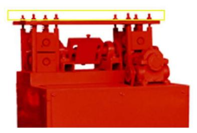
• Adjust the straightener roller, until it has a good straightening performance,
